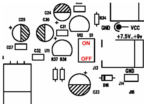
Diagram 3.3 On/Off position of power switch
