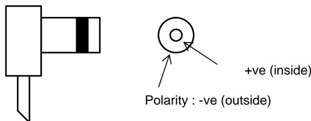
Diagram 3.2 Polarity of DC Jack
