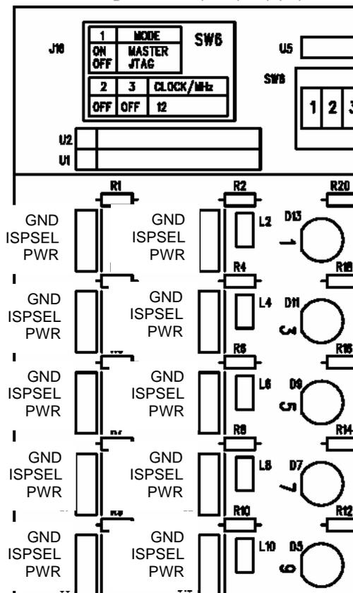
Diagram 4.2 Pin assignments for each connector 'J1' - 'J10'
