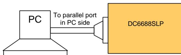
Diagram 3.1 Connection between SL Programmer board and PC
