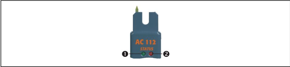
Figure 13: Status LEDs AC112
