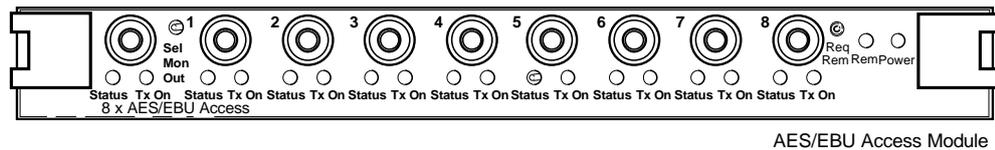
Figure 21. 8 x AES/EBU Access Module
