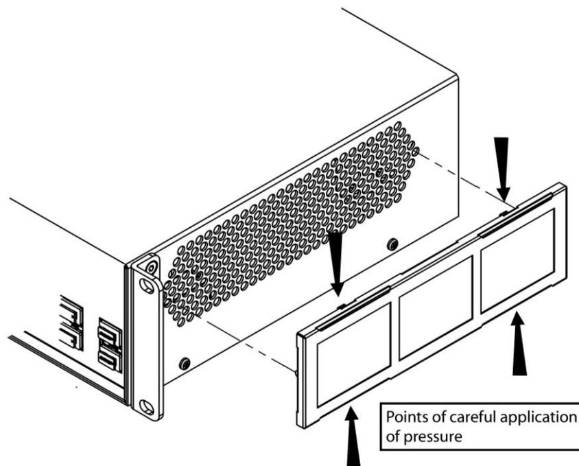
Figure 23. Mounting of external fan filter
