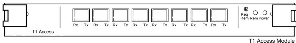
**Figure 12. T1 Access Module**
