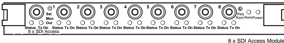
**Figure 19. Front panel, 8 x SDI Access Module**
