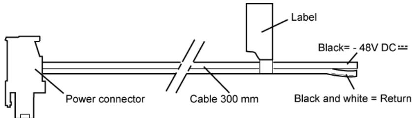
**Figure 22. The power supply cable type NPA0028-0030**
