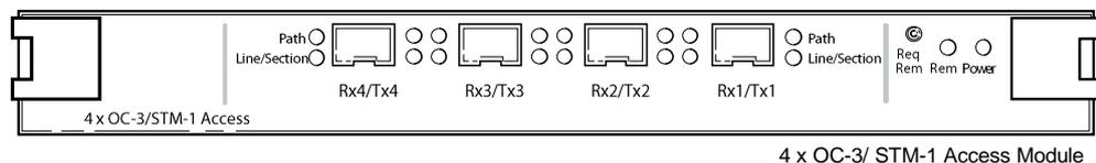
**Figure 15. Front panel for 4 x OC-3/STM-1 Access Module**
