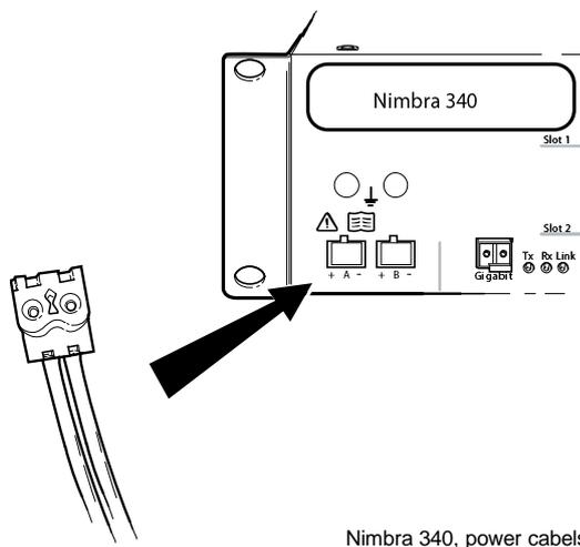
**Figure 24. Placement and front layout of the power inputs**
