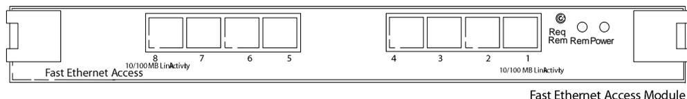
**Figure 13. Fast Ethernet Access Module**
