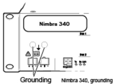
**Figure 25. Placement and labeling of grounding sockets**
