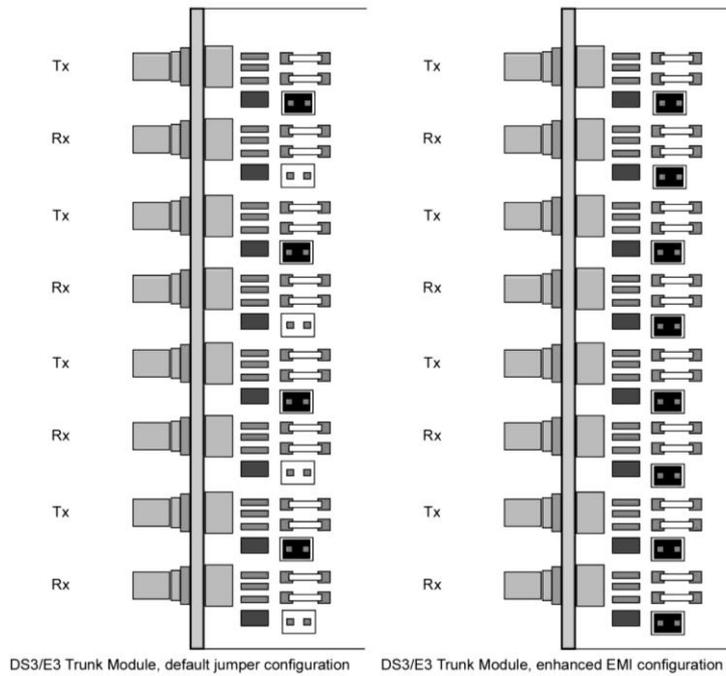
Figure 9. Jumpers settings on the DS3/E3 Trunk/Access Module.
