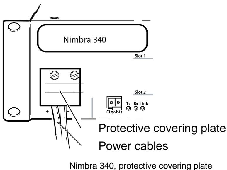
**Figure 26. Placement of the protective cover plate**
