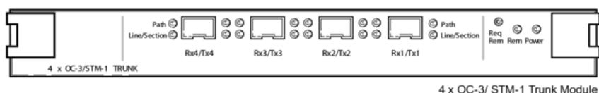
Figure 7. 4 x OC-3/STM-1 Trunk Module
