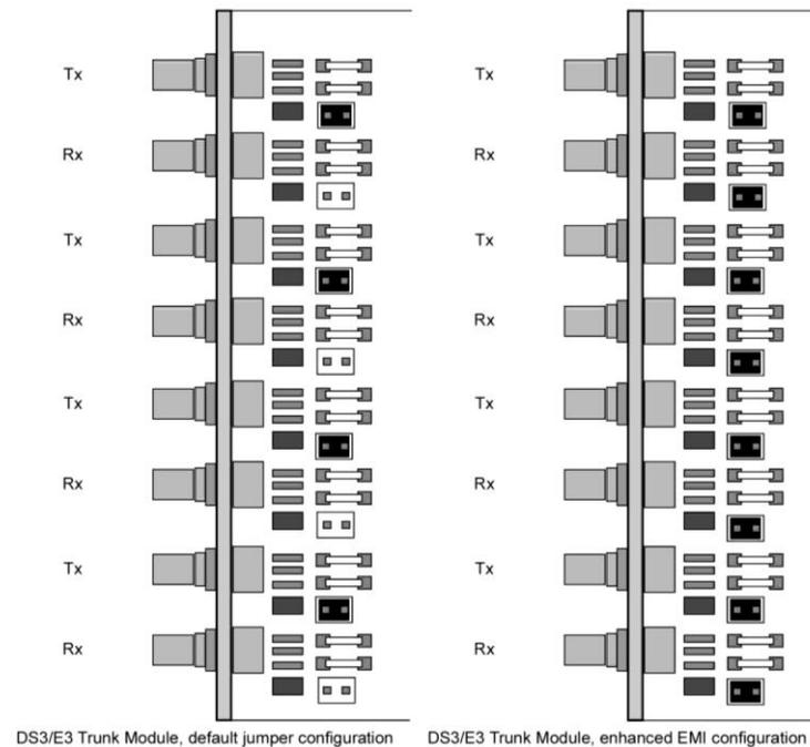
**Figure 17. Jumpers settings on the DS3/E3 Trunk/Access Module.**
