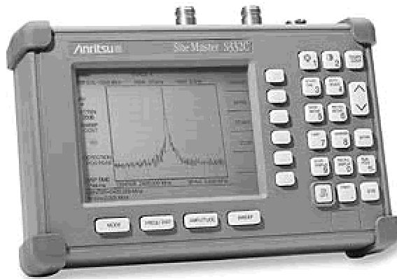
FIGURE 9.12 Picture of a handheld digital spectrum analyzer showing a narrowband signal
