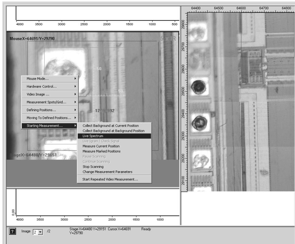
Figure 47: Activating the Live Spectrum Mode
