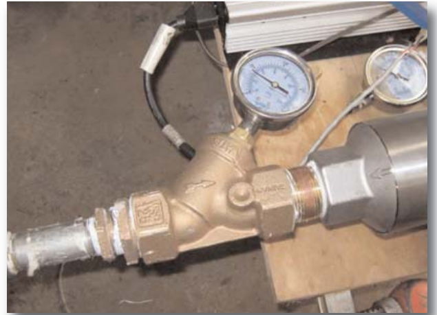
Figure 2-4 Water Supply Connection
