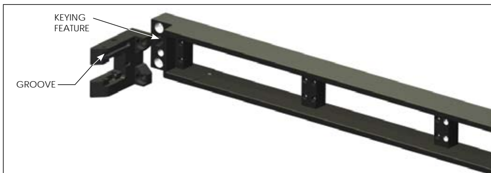
Figure 11-B. The rotation blocks were also designed with a tongue and groove feature to prevent placing the ITA in backwards.
