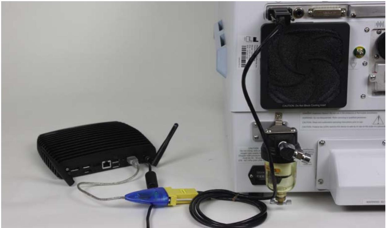
**Figure 5-1** Typical attachment of VIK to Ventilator
