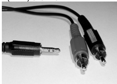
Stereo mini-jack (left), RCA jacks (right)
