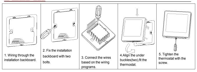
Note: Be sure to connect all the wires as per the wiring diagrams and keep it away from water, mud and other material so as to prevent the unit being spoiled!
