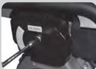
Fig.7 Untight screw of air filter cover
