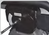
Fig.7 Untight screw of air filter cover
