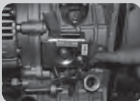
Fig.18 speed handler at STOP position
