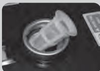
Fig.29 prime fuel filter soundproof type
