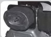
Fig.8 Air filter element
