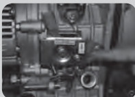
Fig.18 speed handler at STOP position
