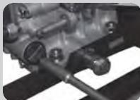
Fig.24 prime oil filter screw
