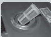
Fig.30 prime fuel filter open type
