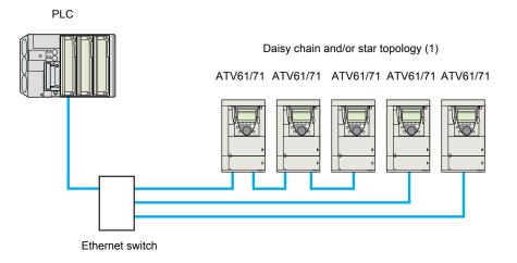
(1) When the topology is a daisy chain, if one drive is turned off, the other drive(s) stop in response to a communication network fault (CNF). Redundancy can be added by connecting the first and last drive in the daisy chain to a hub or switch to create a loop.
