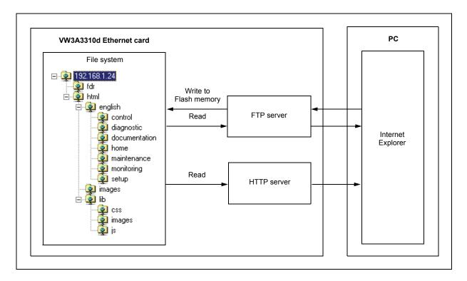
The Ethernet card has an embedded FTP server which authorizes access to the various URLs available for the HTTP server. A browser such as Internet Explorer can be used to display the URLs like a disk in the Windows explorer. This "disk" consists of various directories containing the URL files. It is therefore possible to use the different commands managed by Windows explorer such as deletion, renaming or writing (downloading) files (check that card IO Scanning has been disabled).
