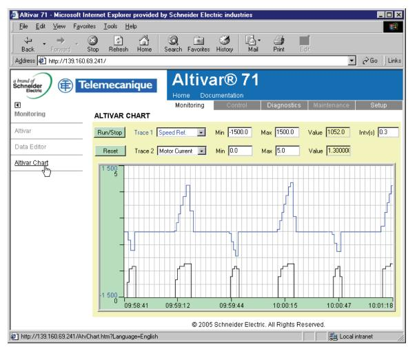
Two parameters can be selected and displayed simultaneously. To do this, select them in the **Trace1** and **Trace2** list.
