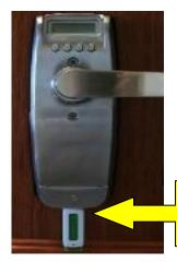
12b) Plug Flash Drive into the USB port located at the bottom of the Interior Unit
