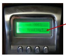
12j) While data is being uploaded from Flash Drive to the ThumbLock® the message, "REC READING" appears on the LCD.
