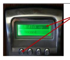
14e) Press the DOWN ARROW until Option 3. U-DISK OP is highlighted.
