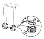
1. Open the door that needs to be adjusted and loosen the clamping nut (A) at the bottom of the door by turning it clockwise ( ) using the spanner included in the product package. (Raise the lower of the two doors first.)
