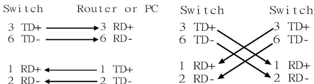
Figure C Straight Through Cabling Schematic Schematic
