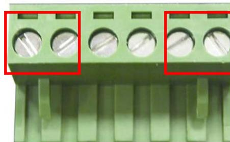
2. Tighten the wire-clamp screws to prevent the DC wires from being loosened.
