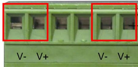
1. Insert the positive and negative wires into the V+ and V- contacts respectively of the terminal block connector
