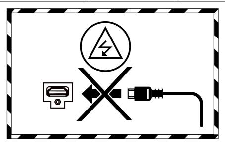
Prior to connecting any device to this unit, switch the projector in standby mode. Never connect a HDMI source to this unit when the projector is in operate mode. The HDMI termination is a self-powered connection and can cause electric discharges.
