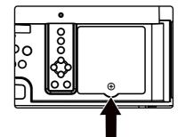
• Open the lamp Cover and loosen the 2 screws on the lamp unit to release it.
