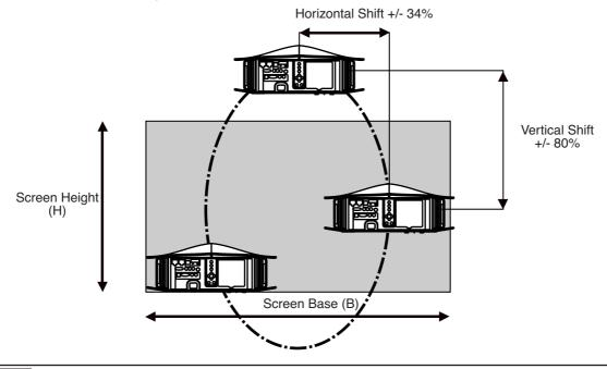
This unit comes with a vertical and horizontal shift to suit most installations. Make sure that your installation does not exceed 80% vertical offset and 34% horizontal offset to avoid trapezoidal correction.
