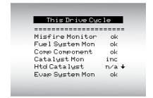
Abbreviations and names for OBD II Monitors supported by the Scan Tool are shown below. They are required by the United States Environmental Protection Agency (EPA). Not all monitors are supported by all vehicles.
