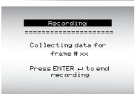
✓ Scan Tool recording times vary. A recording consists of frames of data prior to trigger and several frames after trigger.
