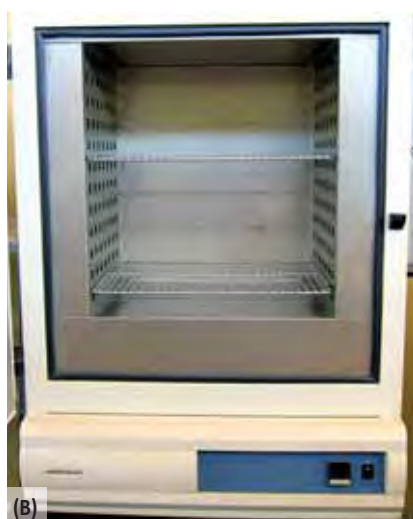
Figure 22.1. Drying ovens: (A) large capacity forced-draft oven; and, (B) small capacity non-draft oven (suitable for drying open container samples; e.g., soil moisture samples).
