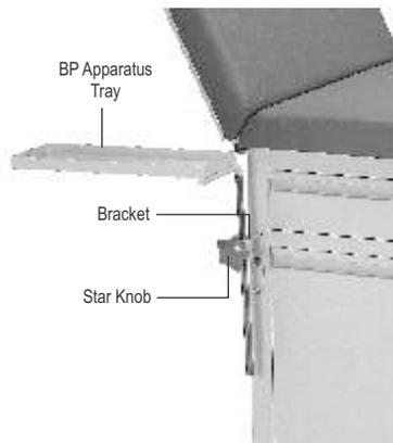
2. Insert the BP Tray Holder Rod into the bracket & tighten the same with the help of Star Knob
