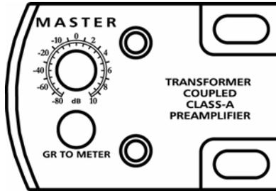
**MASTER (LEVEL):** This control adjusts the output level of the EUREKA. It functions as a master fader for the entire processing strip. It is useful for adjusting the overall output level up or down to match the optimum input level of a recorder, mixer, etc.
