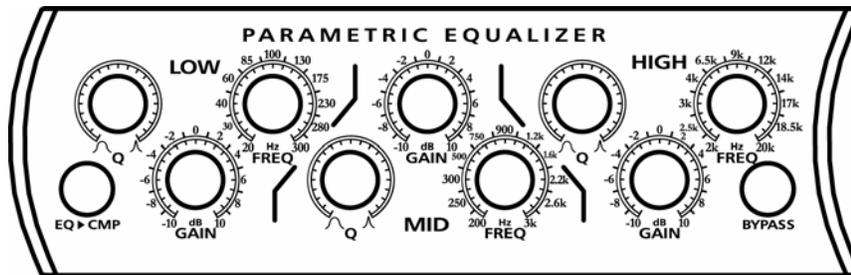
The EQ is divided into three sections or bands (Low, Mid and High) Each band has the following controls:
