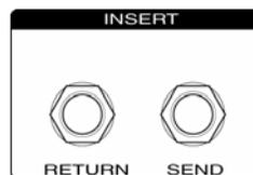
The EUREKA features ¼” TRS balanced **Send** and **Return** jacks. These connectors allow the use of external processors such as reverbs, de-essers, limiters, EQ’s, etc. Simply connect the send jack, balanced or unbalanced to the input of the external processor. Then connect the EUREKA’s return jack to the output of the external processor. The signal is now routed out of the EUREKA,
