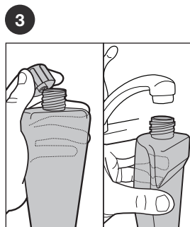
Turn Cap counterclockwise to remove. Fill tank with water.
