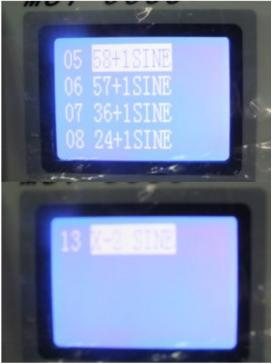
Select one ECU type to enter in, display change ECU output frequency (i.e.speed)adjustable range from 0020 to 2160 Hz, adjust by + and —, signal output end is +B (power), GND( ground wire), CKP (crankshaft speed signal), A1, A2, +,+,B1.B2, stepping motor signal output end.
