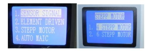
The fourth option, the entire vehicle simulation signal AUTO MAIC, select second option universal car signal simulation. ( or directly select F1, into the universal car signal simulation)
