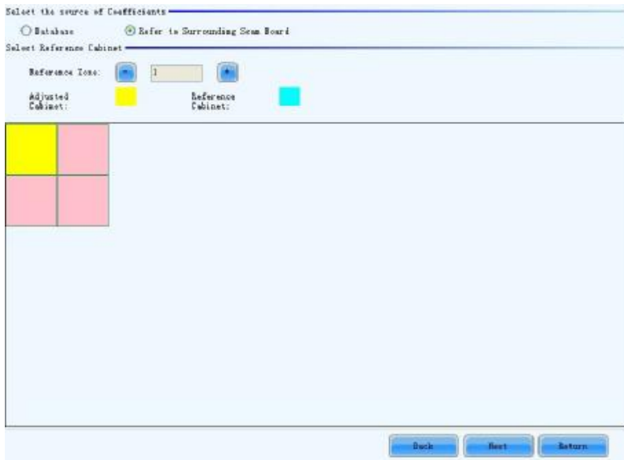
Fig.4.8.11 the page for generating coefficients for the new receiver card according to those of its surrounding receiver cards
