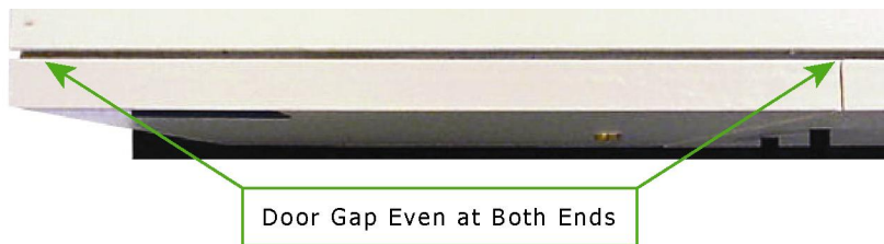
Figure B.1 - Top View of SAC with Properly Sealed Door
