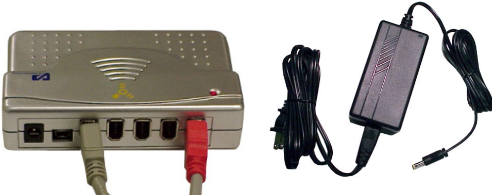
Figure 1.6 - Fire Wire Hub with Cables and Inverter
