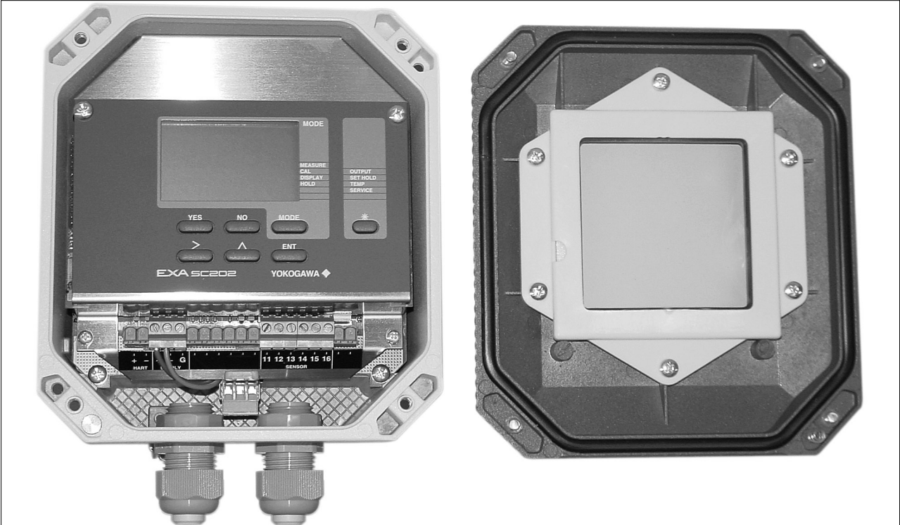
Figure 3-4. Internal view of EXA wiring compartment
