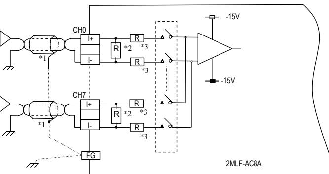
\*1) Use the cable of 2-core twisted shield. AWG 22 is recommended for the cable standard.
