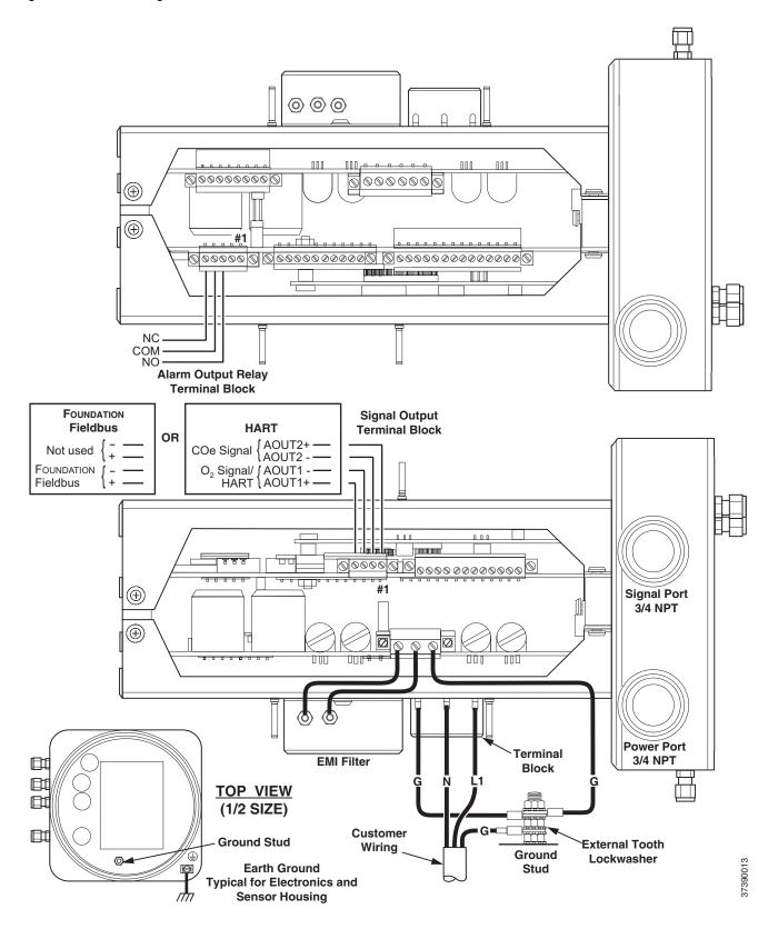
Figure 2-7. Electrical Connections Between Remote Electronics and Sensor Housing GRN **\\\\\\**#1 YEL 2HTR CO <del>0</del> RED 1HTR CO 0 BLK 2HTR O, 0 ORG 1HTR O 0 То WHT 2HTR SB ground 1HTR SB screw **Heater Power** Connector (J3) 000 000 000000000 000000  $^{\oplus}$ **( RED** T/C CO+ T/C CO-00000 BLK WHT T/C SB+ BLK **Heater Power Cable** T/C SB-GRN YEL T/C O2+ BRN O EXC+ BLK T/C O2-CO ACT+ BLK 0 BLU CO ACT-O2 CELL+ **COe Sensor** 0 and O2 CELL-RED CO REF+ CO REF+ Cold Junction
