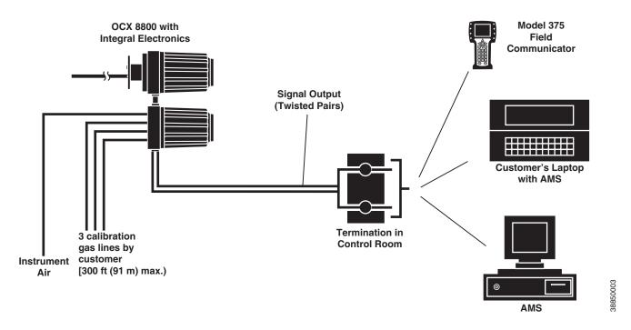
Figure 1-4. Communication Connections and AMS Application - OCX 8800 with Remote Electronics
