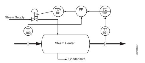
Figure 7-18. PID Function Block Diagram for Feedfoward Control
