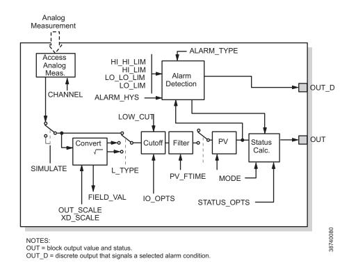
Figure 7-7. Analog Input Function Block Timing Diagram
