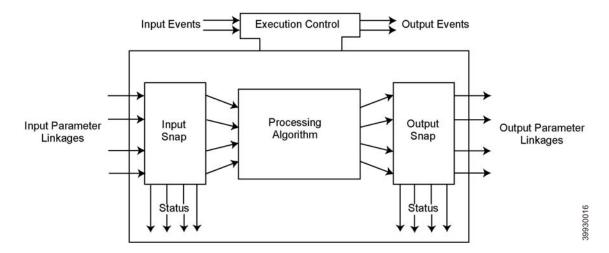
A block is a tagged logical processing unit. The tag is the name of the block. System management services locate a block by its tag. Thus the service personnel need only know the tag of the block to access or change the appropriate block parameters.
