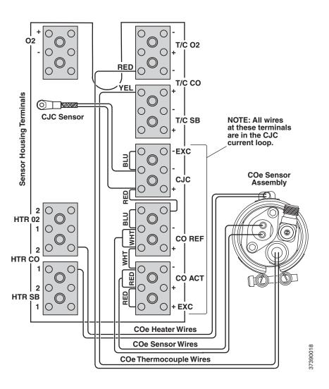
Figure 9-10. Removal of COe Sensor Assembly
