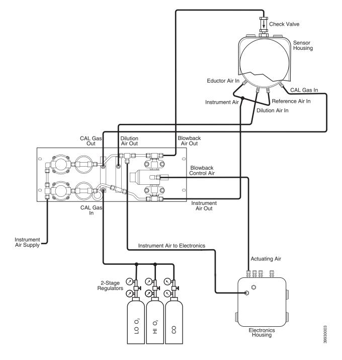
Figure 2-16. Pneumatic Installation, Blowback Panel with Autocalibration without COe Zero Function
