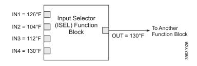
Figure 7-29. Input Selector Function Block Application Example (SEL\_TYPE = avg.).
