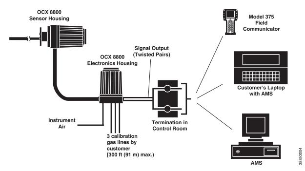
Figure 1-5. Typical System Installation - Integral Electronics
