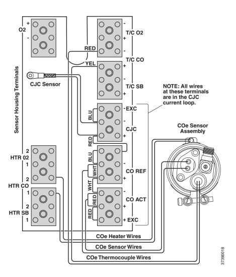
Figure 9-22. Installation of  ${\rm O_2}$  Cell and Heater Strut Assembly
