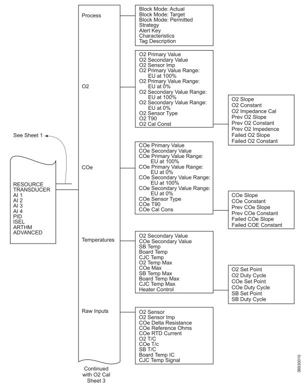
Figure 6-9. Fieldbus Menu Tree (Sheet 3 of 3
