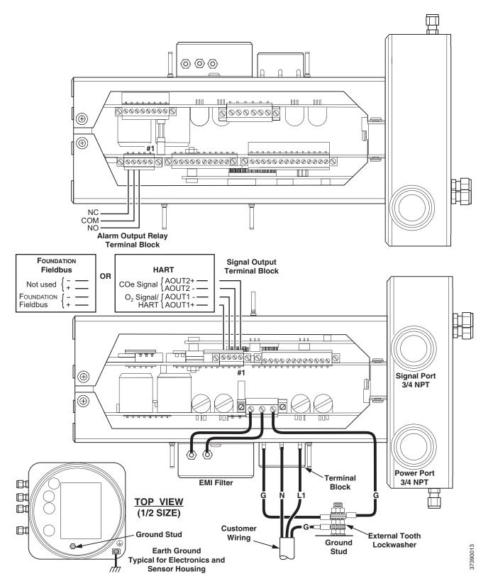
Figure 9-6. Remote Electronics Housing Cable Connections
