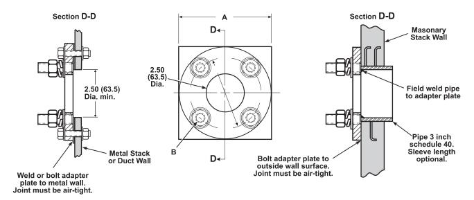
METAL WALL STACK OR DUCT CONSTRUCTION
