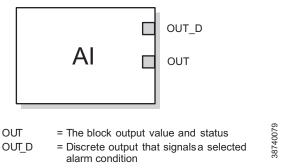
The Analog Input (AI) function block processes field device measurements and makes them available to other function blocks. The output value from the AI block is in engineering units and contains a status indicating the quality of the measurement. The measuring device may have several measurements or derived values available in different channels. Use the channel number to define the variable that the AI block processes.
