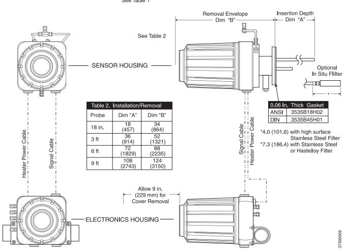
Figure 2-3. Adapter Plate Installation
