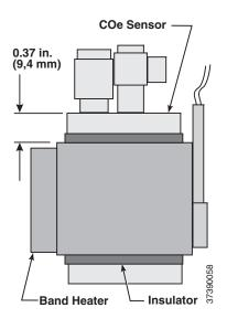
Figure 9-20. COe Sensor Holder Alignment
