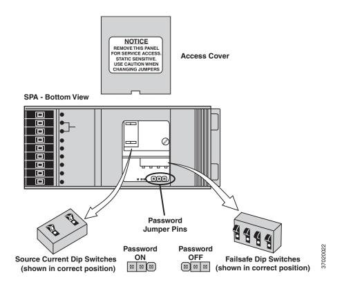
Figure B-4. SPA Setup for Calibration
