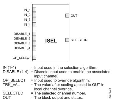
The Input Selector (ISEL) function block can be used to select the first good, Hot Backup, maximum, minimum, or average of as many as four input values and place it at the output. The block supports signal status propagation. There is no process alarm detection in the Input Selector function block.
