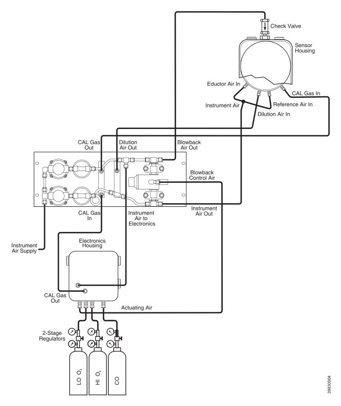
Figure 2-17. Pneumatic Installation, Blowback Panel with Autocalibration with COe Zero Function
