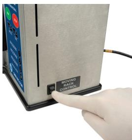
Note: If stationary operation is desired, load the tube holders as described in section 2.1 and leave the processing rack toggle switch in the Off position during processing.
