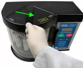
**CAUTION:** The lever should move with smooth and constant motion. If the lever does not slide smoothly as it is moved to the right:
