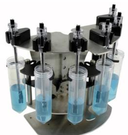
**CAUTION:** DO NOT allow Omni Tips/Stainless Steel Probes to touch the bottoms of the tubes.
