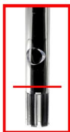
**PLEASE NOTE:** Portion of Omni Tip/Stainless Steel Probe shown below the red line must be submerged in liquid during processing.
