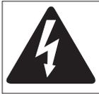
This symbol is used to warn operators that uninsulated "dangerous voltages" are present within the equipment enclosure that may pose a risk of electric shock.
