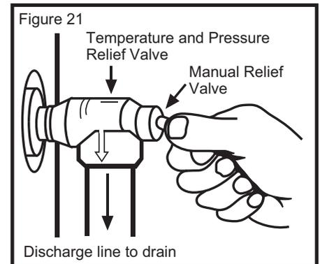
drain. Standing clear of the outlet (discharged water may be hot), slowly lift and release the lever handle on the temperature and pressure relief valve to allow the valve to operate freely and return to its closed position. If the valve fails to completely reset and continues to release water, immediately shut off the manual gas control valve and the cold water inlet valve and call a qualified person.
