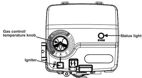
**IMPORTANT:** If the pilot will not stay lit after several tries, turn gas control/temperature knob to "OFF" and check the status light for flash codes. Record any codes and call your service technician or gas supplier.
