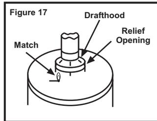
If the flame flutters or is blown out, combustion products are escaping from the relief opening. If this occurs, do not operate the water heater until proper adjustments or repairs are made to the vent pipe system and/or air supply requirements.
