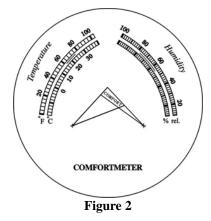
The calibration and positioning of the hands are designed to indicate perfect comfort conditions in room atmosphere: when both hands cross in a limited area of the dial, or the "COMFORT zone".
