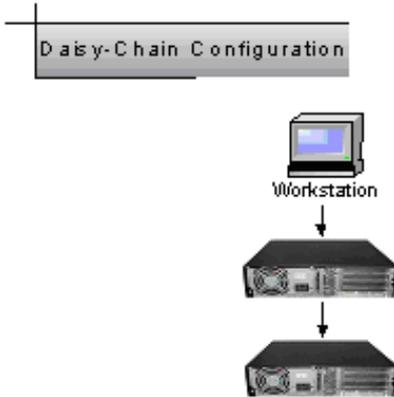
In the daisy-chain configuration, successive PCIe expansion systems are added to the "end" of the PCIe expansion hierarchy, which adds "depth" to the Local Bus by increasing the number of the logical PCI levels active in the system configuration.
