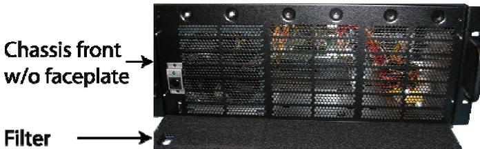
Finally, replace the filter and faceplate. Secure faceplate with four Phillips screws. Tighten screws until snug. Turn on power to the chassis.
