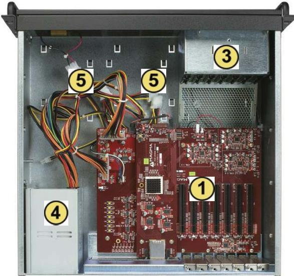
Be sure to keep the can of compressed air about six inches from the parts being sprayed with air. Pay particular attention to the fans in the chassis **2** and power supply **3** because they are critical to air movement and to keeping your chassis cool. Also spray the PCIe slots **1** on the backplane, and the chassis bay areas **4**. If you have mounted hard drive cages in one or both of these areas, be sure to check for dust that can collect in the space between the drives.
