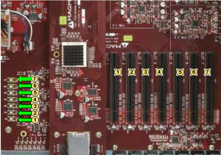
Simply press the button corresponding to the slot you wish to “power-down,” hold the button for a minimum of five (5) seconds and then release it. The power has now been removed from that slot. All other PCIe cards remain fully functional, as they are independent of this slot.
