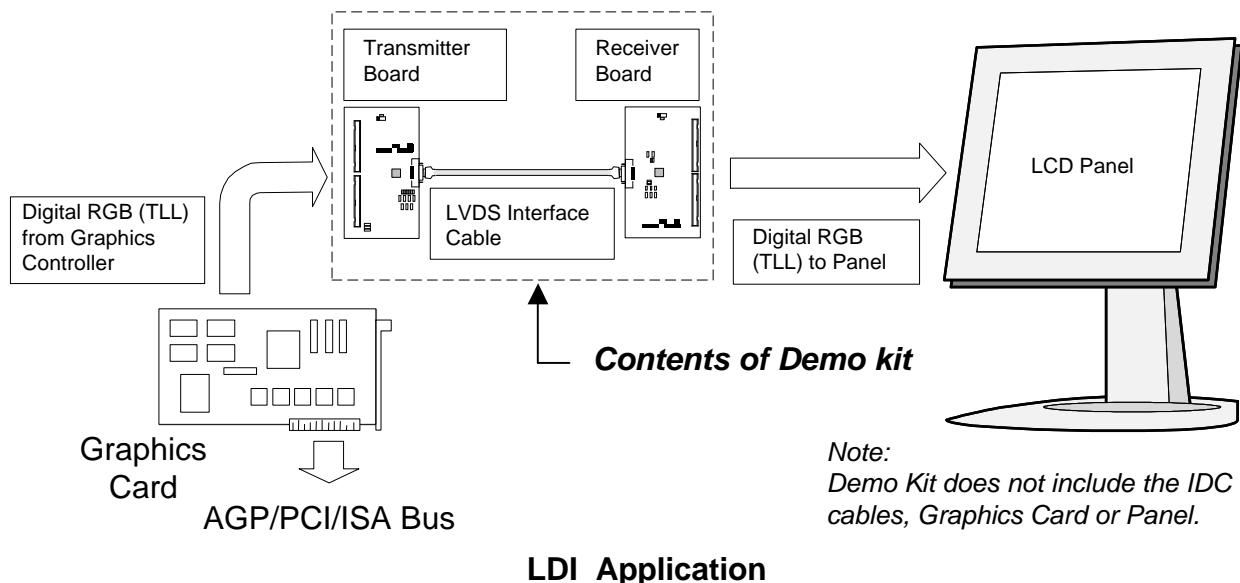
The diagram above illustrates the use of the Chipset (Tx/Rx) in a Host to LCD Panel Interface.
