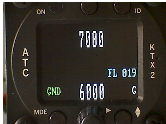
GND-switch installed, on GND
