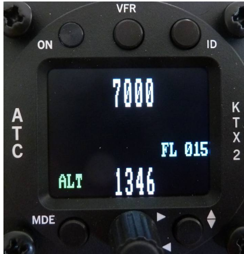
No GND switch installed
