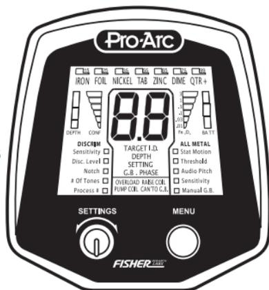
When manually ground balancing, try to “feel out” a spot on the ground to make sure there is no metal present. In order to avoid locking onto metal, the computer will not balance to ground where the GB setting is less than 40. Where the ground reads less than 40, manual ground balancing is required.
