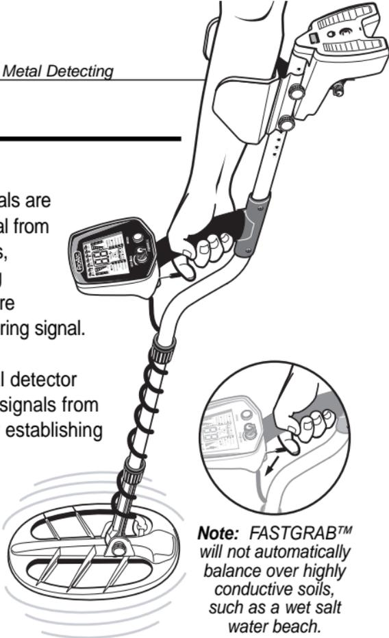
**Note:** FASTGRAB™ will not automatically balance over highly conductive soils, such as a wet salt water beach.
