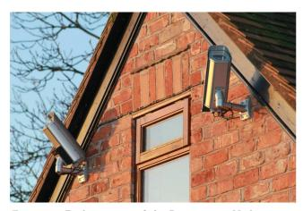
Figure 1 – Both cameras of the Ravensmoor Node permanently affixed to the gable end of a brick building. The unit on the left faces east while that on the right faces north. Note the black spacer block on the left hand unit between the camera housing and the mounting bracket. This modification was required in order to allow the appropriate elevation to be achieved without the rear of the housing fouling on the horizontal support bracket.
