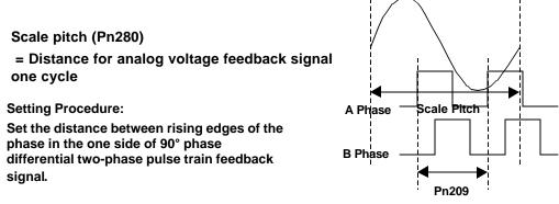
The distance 1/4 of the linear encoder resolution (Pn209) is controlled as a minimum feedback pulse in the servo amplifier.
