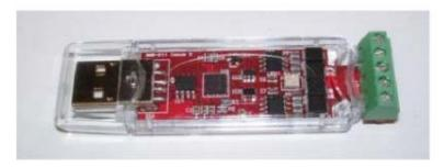
The MIC-USB485CVTR should be connected to the telemetry header (HD5) of the MIC power supply with Standard Twisted Pair cable such as Belden 8760.
