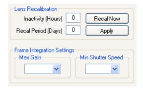
This section defines when and how often the Sony Optical Camera block should perform a recalibration process. The first field Inactivity defines how long in hours it should be after the last manual control command before the first recalibration should take place, and the second is a time in days between each successive recalibration from then on.
