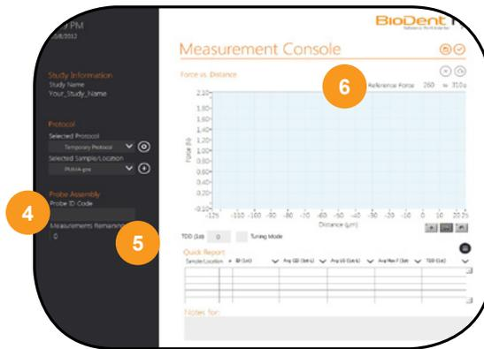
5. **Measurements Remaining.** Displays the number of measurements remaining for the Probe ID code entered.
