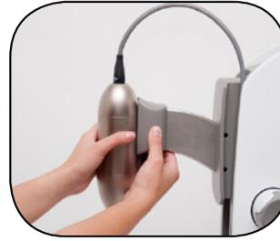
While pressing button, either raise or lower MHU into position 1 (for larger/taller samples) or position 2 (for smaller/shorter samples). Release button to lock position.
