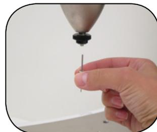
While holding the Probe Assembly by the square hub, insert the top of the Test Probe into the opening of the Measurement Head Unit (MHU); there is an automatic magnetic attachment you will feel if inserted correctly.
