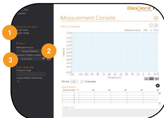
4. **Probe ID Code.** Displays the ID code you entered corresponding to the probe you will be using.
