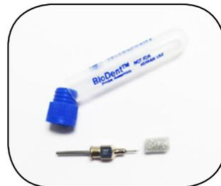
With the Test Probe and the Reference Probe coupled, hold the Probe Assembly by the Reference Probe's square hub.
