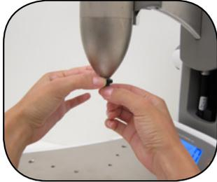
Hold the black wheel still with your free hand. As you push the Reference Probe up, ensure the Reference Probe engages the thread. Once it does, gently twist it counter-clockwise until finger tight.
