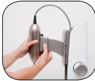
Press button with your right thumb to release the MHU positioning lock.
