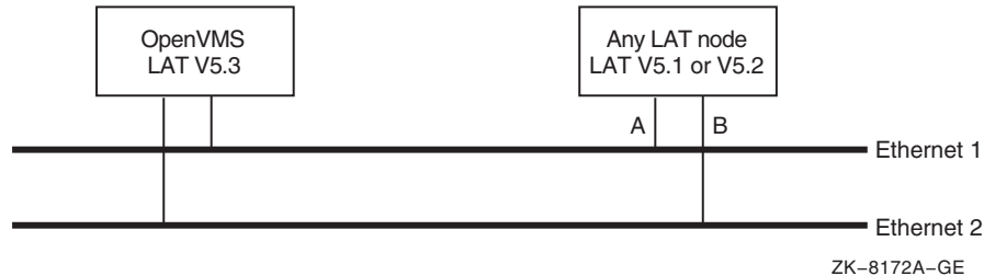
Figure 26–5 Unsupported Multiple Address LAT Configuration
