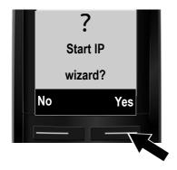
> Press the key below Yes on the display (= right display key).
