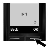
The configurable IP connections are shown in the following displays (IP 1 to IP 6). VoIP connections that are already configured are marked with ☑.
