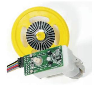
Incremental quadrature encoder system for gearhead motors
