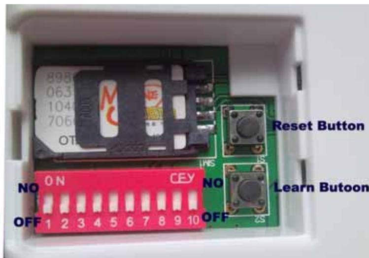
After this operation, all the added wireless detectors and wireless panic buttons will be removed from the control panel, and all of the settings will be reset to the factory default.
