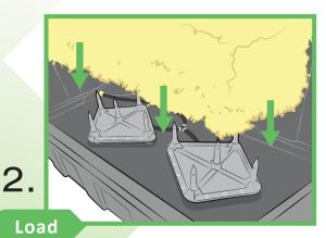
Place bale or loose hay over Steam Manifolds and **push down firmly** so Manifold Spikes pierce hay to their full length. Lower Lid and fasten Catches.
