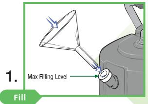
Use funnel and watering can provided to fill Steam Generator until water is visible in Filler Spout.
