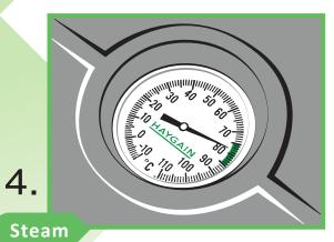
Allow hay to steam for **at least 50 minutes** and Lid Thermometer reads in green band **above 80° centigrade** for at least 5 minutes.
