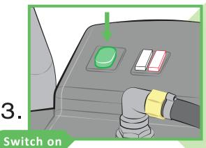
Push down green On/Off Button located on top of Steam Generator.
