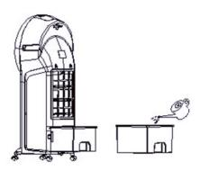
3. Replace the tank back onto the back of the unit. Turn the water tank knob clockwise 90°. This locks the water tank back into place.
