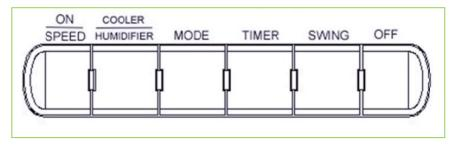
After the tank is filled with water, connect the evaporative cooler to a power outlet. The unit will beep twice, indicating that the power source is connected. The cooler will be in standby mode at this time.
