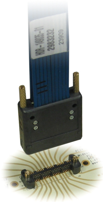
Figure 5.2: Cable Connection to PCB Connector
