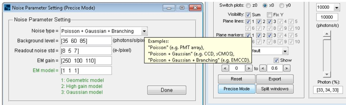
**Figure 7.4.1: Entering the noise parameters**
