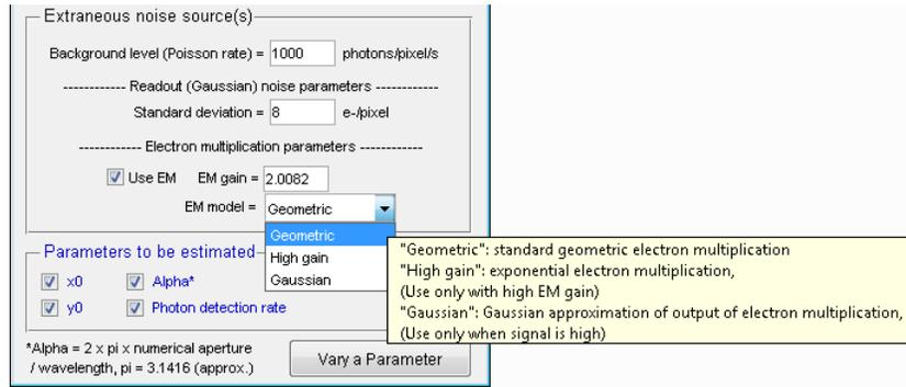
**Figure 1.2.3: Electron multiplication parameters**
