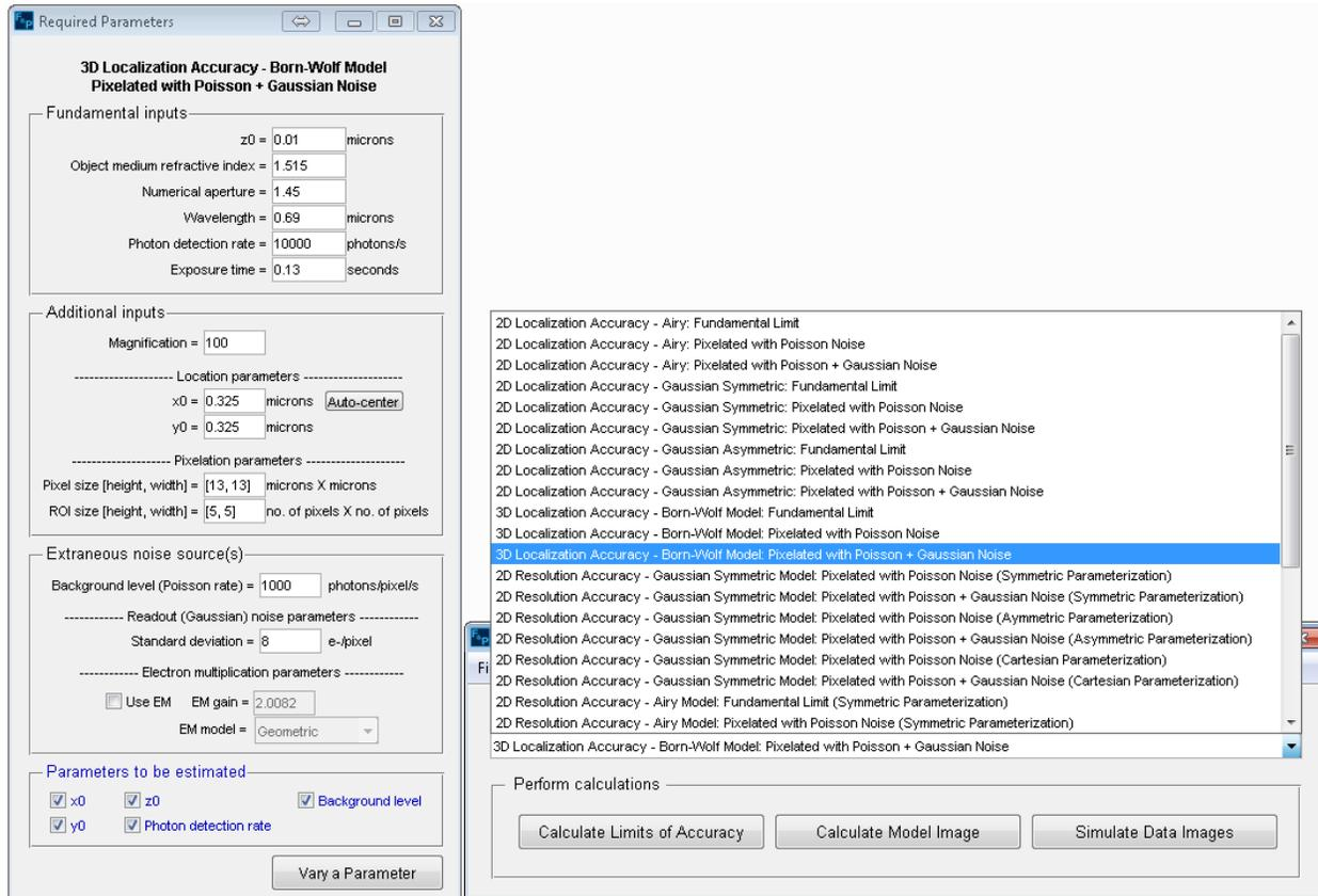
**Figure 8.2.1:** 3D Localization Accuracy problem scenario and its required parameters window
