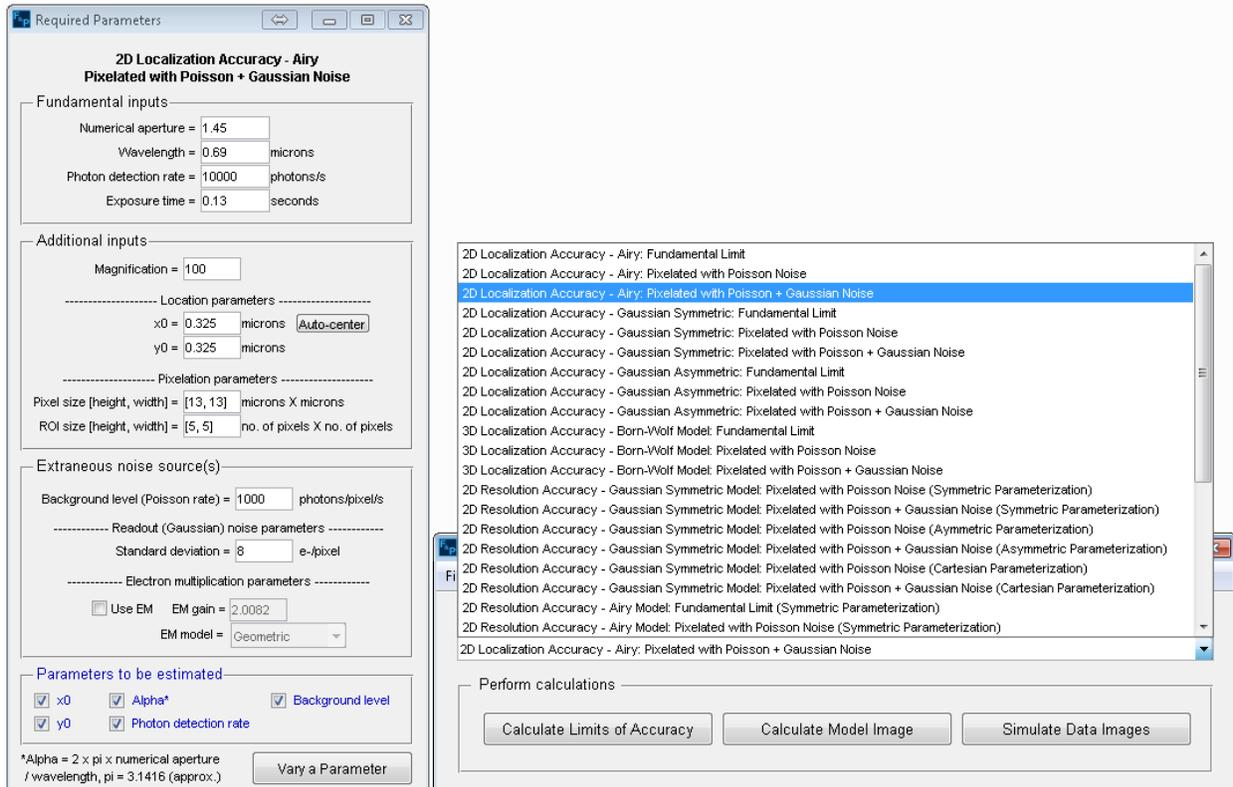
Figure 1.2.1: Selecting the 2D Localization Accuracy calculate type
