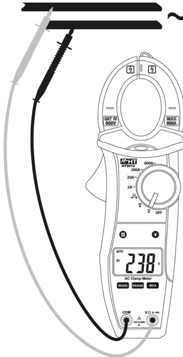
Fig. 4: Taking AC voltage measurement
