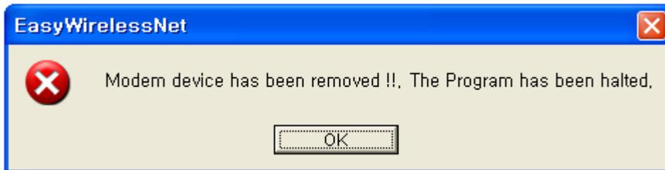
A: The actual connection of USB modem and computer has been disconnected. Please check whether the cable is dismounted, cable is disconnected or USB modem power has been turned off. Then try to reconnect the modem.
