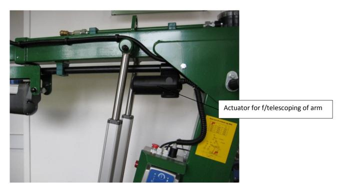
Here, too, all lines should be undamaged, and placed correctly at lead-ins etc.
