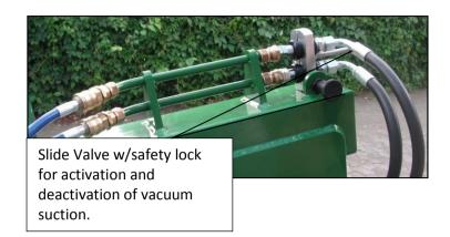
Vacuum suction on both pressure gauges to be 0.62 (between 0.6 - 0.7)
