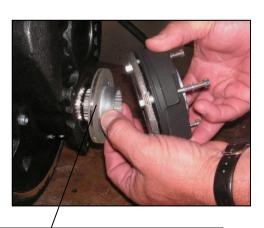
Loosen the 3 bolts on the brake. Carefully remove the "cover" on the brake, and then release the disc. Mount the 3 bolts again, and test.
