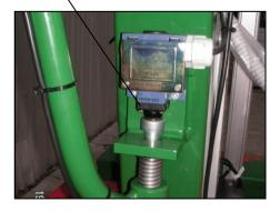
If —no response when pushing control panel, <u>individual functions</u>, Has the safety switch been activated? If activated, try one of the possibilities above. There may be a fault on actuators for movements, or when controlling these.
