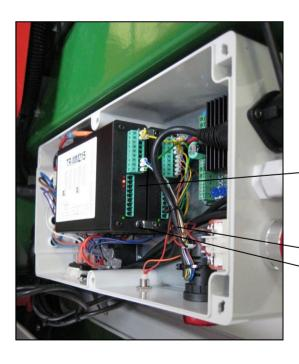
On control box for lift arm actuator. LED No. 7 on when lift arm is down all the way. If LED is on at some other time, there will be a fault at actuator.
