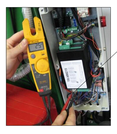
Supply voltage to be checked, should always be 25 Volt. At lack of LED light, always check voltage.
