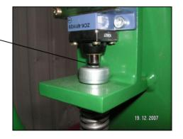
To re-establish function on the machine, you may, for instance, using a screwdriver push up the switch, and the safety switch will resume its function
