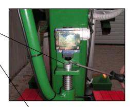
The telescopic arm is run back in, and work too heavy for the machine is lowered back in place. Should the safety switch switch off again at this manoeuvre, you may, using your body weight, push the machine in place by applying pressure on the weight blocks.
